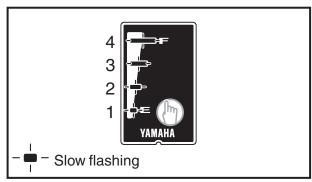
4. If all four battery capacity indicator lamps flash slowly at the same time when the battery capacity indicator button "" is pushed, see "Temperature protection function". (P. 2-14)
