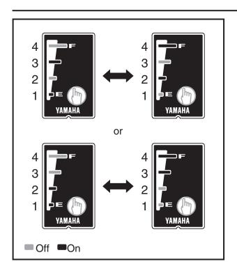
2. If the battery capacity indicator lamps [1]/[3] and [2]/[4] turn on alternately, or the lamps [1]/ [2] and [3]/[4] turn on alternately when the battery capacity indicator button "" is pushed or connect the battery charger, see "Recoverable errors of battery pack or battery charger". (P. 2-8)
