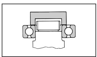
3. When striking a bearing onto an axle, apply a parallel force to the inner race.
