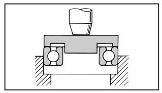
2. When striking a bearing into the case, apply a parallel force to the outer race.
