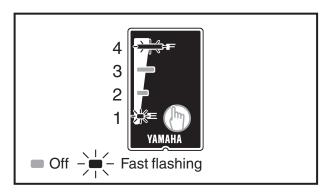
3. If the battery capacity indicator lamps [1] and [4] are fast flash simultaneously when the battery capacity indicator button "" is pushed or connect the battery charger, see "Non-recoverable errors of battery pack". (P. 2-11)
